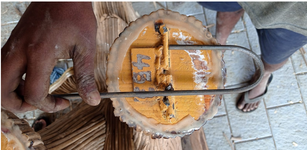
Calf foot has welded in steel loop to attach ground anchors/ chains / Wire
